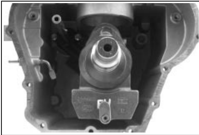
Figure 10-15. Installation du sabot de guidage.
