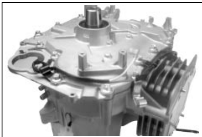
Figure 10-30. Plaque de fermeture en place.
