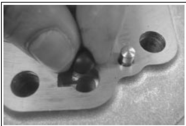
Figure 10-33. Installation du drain.
