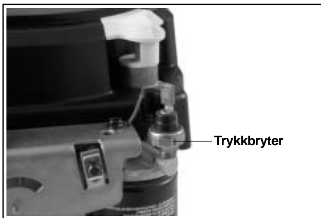
Figur 6-9. Oil Sentry™ Trykkbryterplassering.
